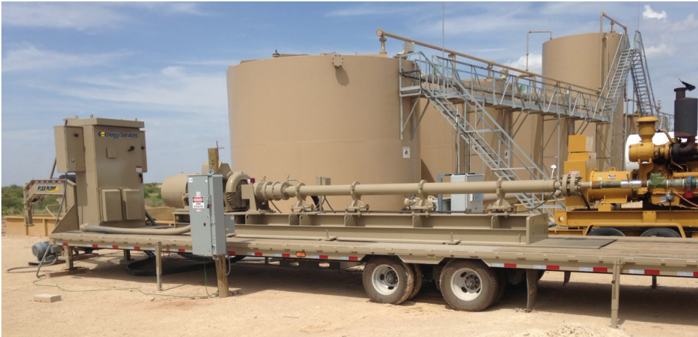
Trailer-mounted horizontal pumping system
