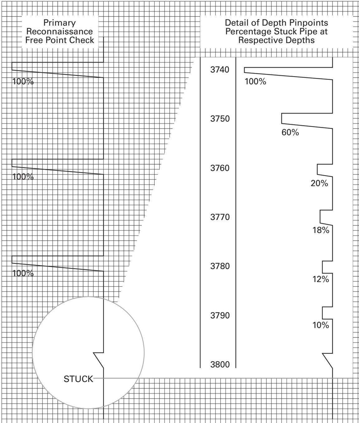
Stuck pipe can be determined by the Motorized Free Point Tool and illustrated so that the operator can determine the ideal depth to perform backoff operations. In this example, the ideal depth would be between 3,740 and 3,750 ft.
