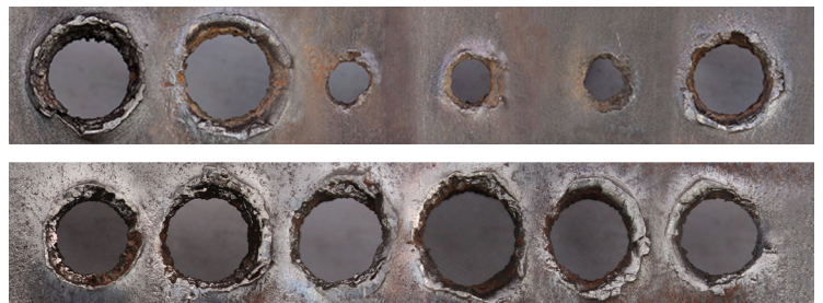
Top: Highly variable entrance hole sizes at 60° phasing, which can cause a 120% drop in near-wellbore pressure. Bottom: Consistent entrance hole sizes, which produce overall improved stimulation results.
